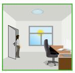
With sufficient natural light, the With insufficient natural light, light does not switch on when presence is detected.
